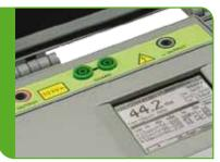
Dot matrix LCD and connector panel for high quality shielded test leads 12 kV (included in standard set)
